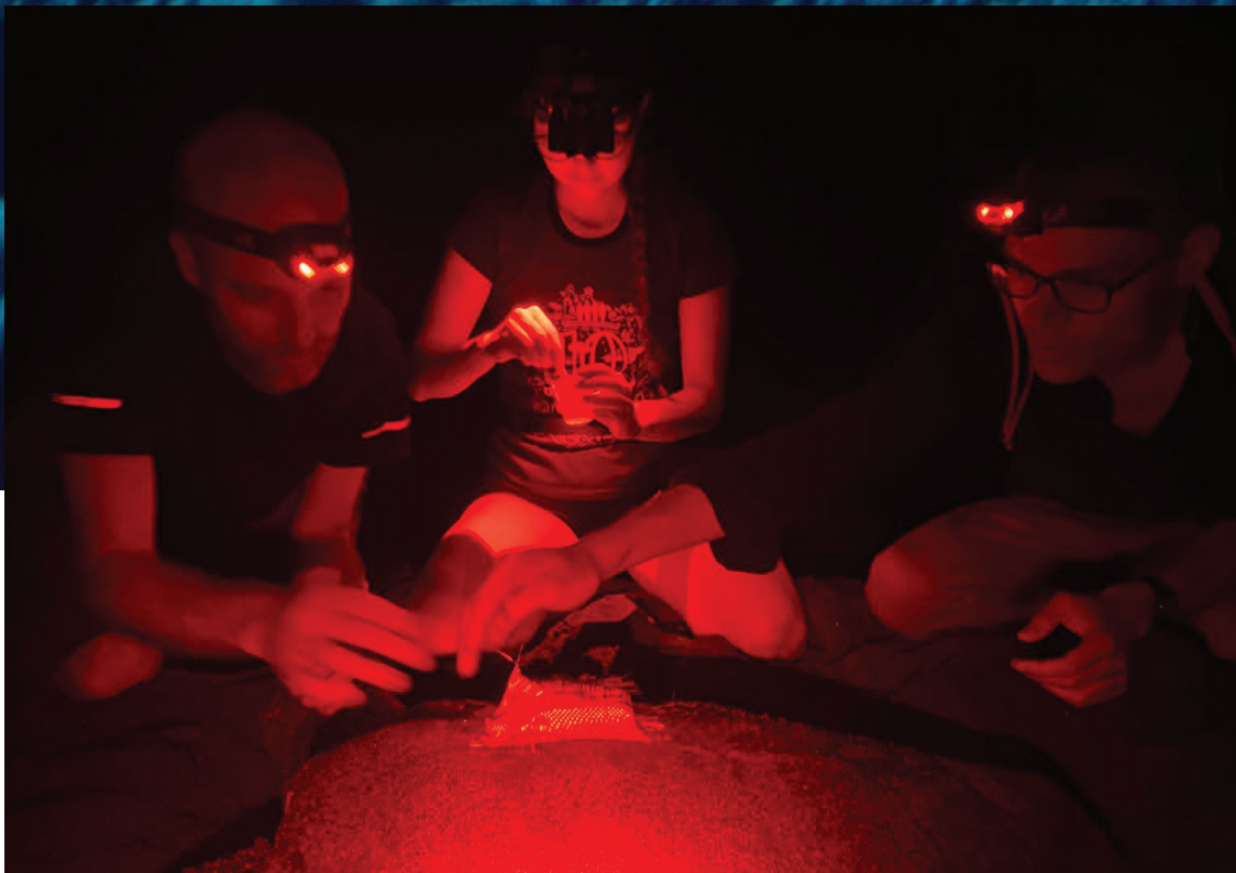
The SnapperGPS tags are glued to the turtle's carapace. The epoxy comes off naturally if the tag is not recovered.
