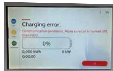
Error message shown by the charging station after the charging session has been disrupted
