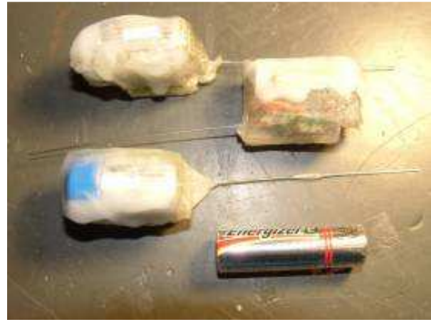
Figure 3. Three spotter class tags. The units have been packaged in epoxy resin for strength and waterproofing. The tags are equipped with a rigid quarter wave whip aerial. An 'AA' battery is shown for scale purposes.
