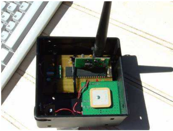
Figure 5. An early prototype pack tag. This tag is equipped with a GPS unit, tri-axial accelerometer, light and temperature sensors.
