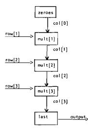
Each process mult[i] inputs a value x from row[i], multiplies it by v[i], adds the product to a partial sum y which it has input from col[i-i], and outputs the result on col[i]. These actions are then repeated.
