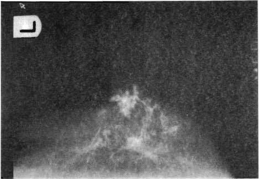
Figure 1.6: The result of removing a constant scatter component from the image in figure (1.1). The removal requires the use of an offset which is set to give an optimal dynamic range.
