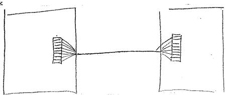
The multilink is a device for multiplexing say eight permanent virtual links through one physical link which connects two transputers.
