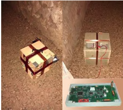
Fig. 10. The two TXs and the RX used in the experiments.
