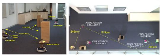
(a) Experimental setup for two localizer configuration. The localizers (with red markers) form a multi-hop distance chain between the sensor robot robot images represent the start positions. (yellow marker) and the anchor (in the far end of the picture).
