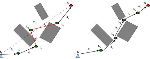
(a) Initial positions of localizers between the anchor and (b) Desired the sensor robot in a cluttered environment. and the sen
