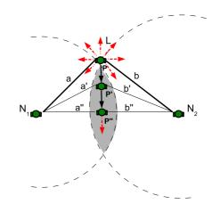
Fig. 4. Alignment procedure of L with neighbours  $N_1$  and  $N_2$ . L chooses the direction (out of  $N_{dir}(=8)$  directions) which offers the maximum decrease in the sum of distances to its neighbours (a+b). The procedure completes when condition (a' + b') < (a + b) no longer holds.
