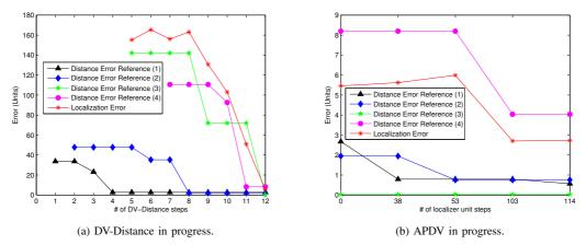
Fig. 7. The sensor robot is initially localized using DV-Distance. The localization error in the cluttered NLOS-prone environment is then further reduced using APDV.
