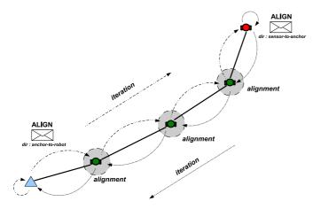
Fig. 3. Working of the APDV algorithm towards refining the distance measurements obtained via initially through the shortest-path-distance search of the DV-Distance algorithm.
