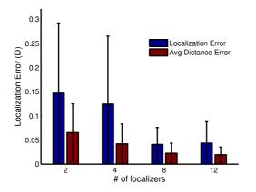
Fig. 9. Effect of the number of localizers on the performance of APDV
