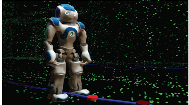
Fig. 1. Localisation against large point clouds comes with a low efficiency and high computational cost making accurate localisation difficult on computationally constrained platforms such as the Nao V5 (with only an Intel Atom @ 1.6 GHz and 48.6 Wh battery). In this paper we reduce the computational load by creating a localisation graph of multiple modalities.
