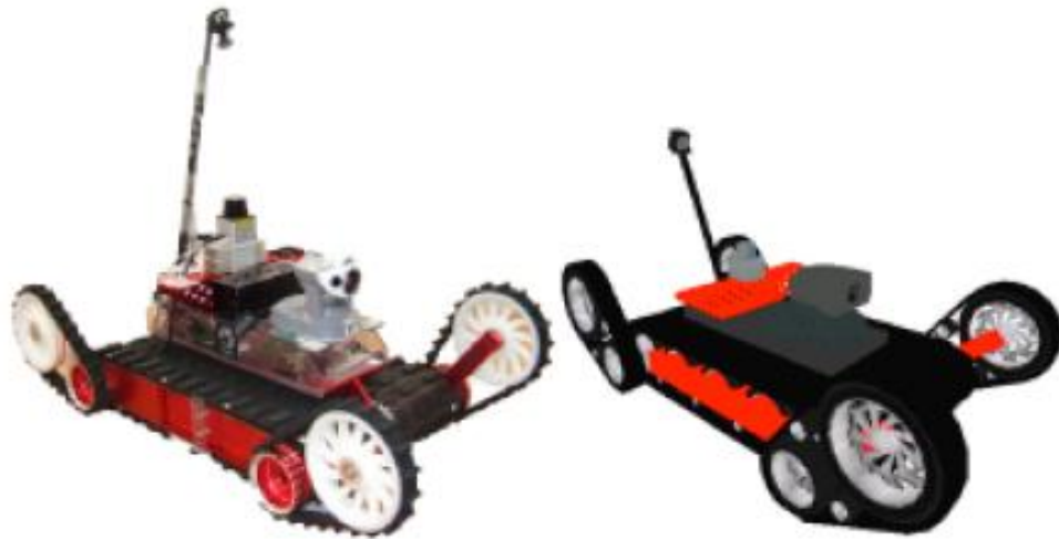
Fig. 1. A real Kenaf robot and its simulated counterpart.
