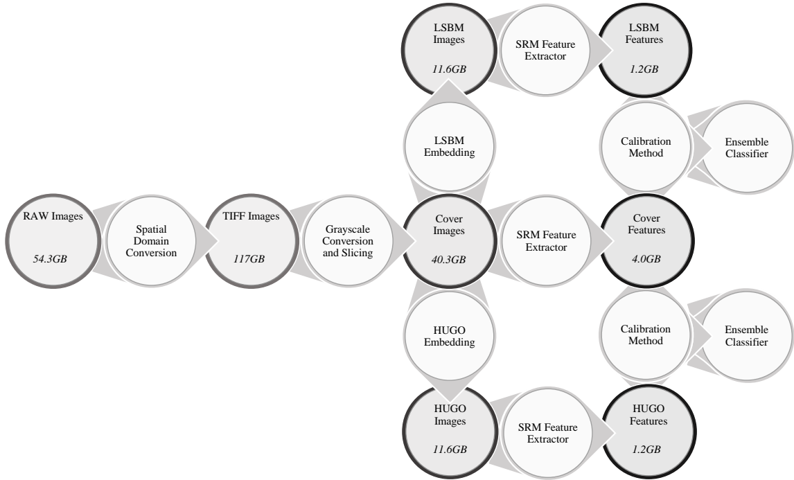
Figure 3.1: Flow chart of the experiment process. As discussed in Section 3.2 the cover sizes (images and features) include all 7 aspects. The LSBM and HUGO embedding was performed on one aspect with two different payloads, creating the image and feature size difference visible in the chart.
